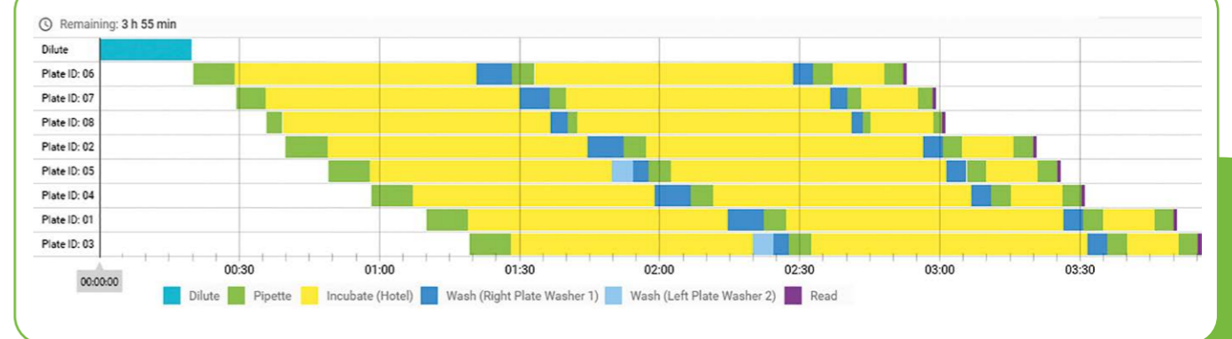
Exemplary workflow with the EUROLabWorkstation ELISA
